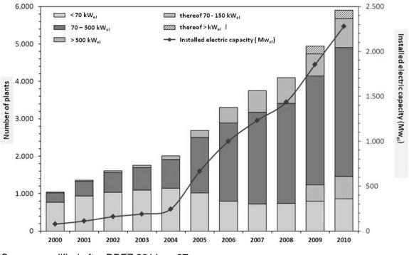
Figure 1: Installed electric power and share of different plant sizes
